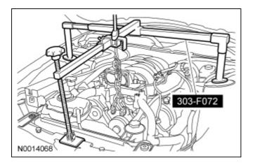
17. **NOTE:** Both the RH and LH engine support insulator nuts must be removed to allow the engine to be raised.
