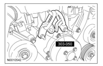
15. If equipped, remove the 4 nuts and the strut tower cross brace.
