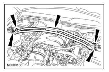
16. Install the Engine Support Bar.
