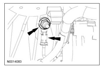
20. If equipped, remove the nut and position aside the transmission cooler tube bracket.
